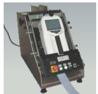
Fabric Continuous Caliper and Air Permeability Measurement
