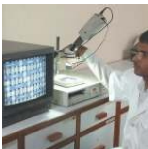
Fabric frame-structure analysis
