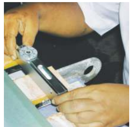
Foil angle measurement on the machine
