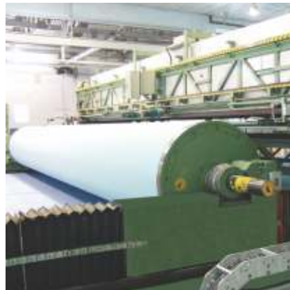
11 M wide-fully PLC controlled, heat setting/finishing table
