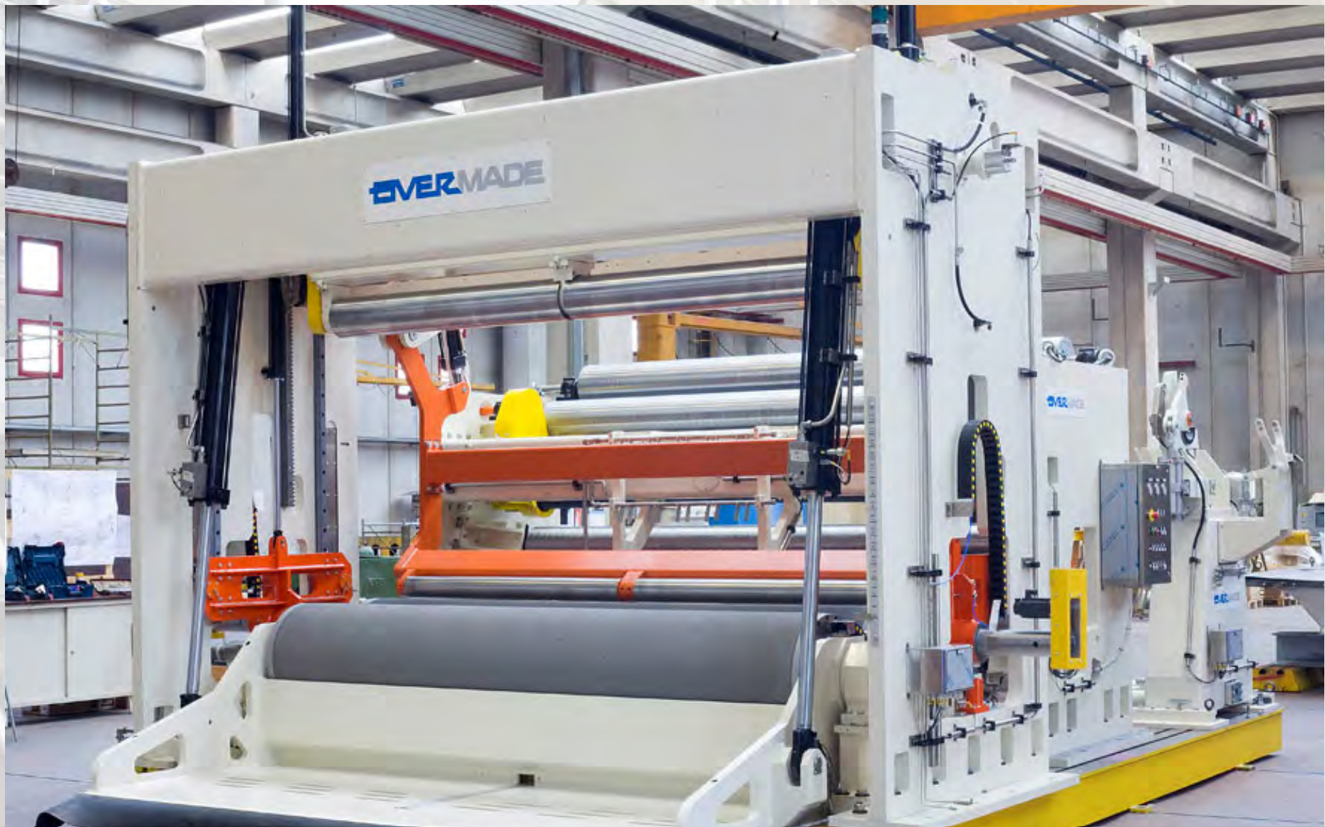
Type: Two-drum shaftless winder Application: MG Paper, up to 2.600 mm and 1.200 mpm
