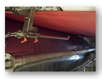
The detector can be easily aligned, the parametrization is done by means of the PC-based user software "TriIdentMaster".
