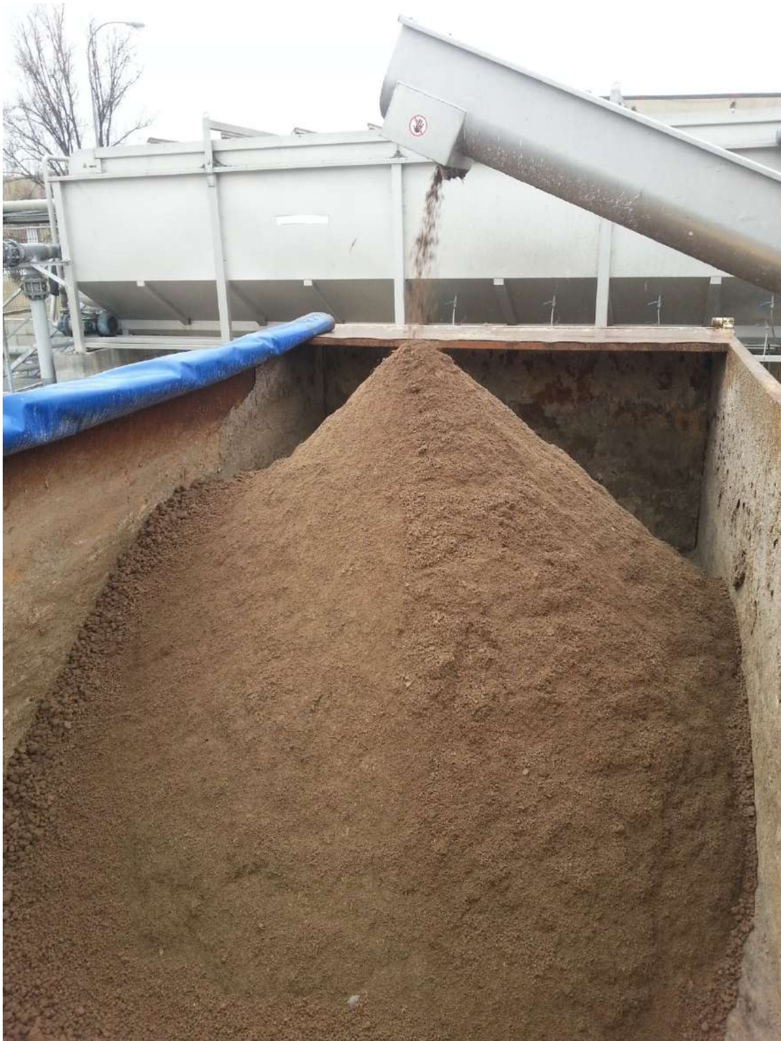
Picture 4 : Previous Thickened of sludge before centrifugation to obtain dried solid and more easy to transport. The dimensión of the Decanter must be tailor size made to obtain the results that we want to achieve in the final parameters of the plant before pouring wáter to the river or municipality..
