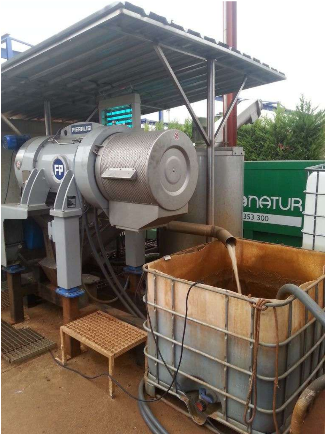
Picture 3 : It's very important the design and measurement of the centrifugation equipment (Decanter) to obtain a clean clarificate that no pollute the inlet flow, otherwise the Project is not good in previous planification and will be problems we it begins to run.
