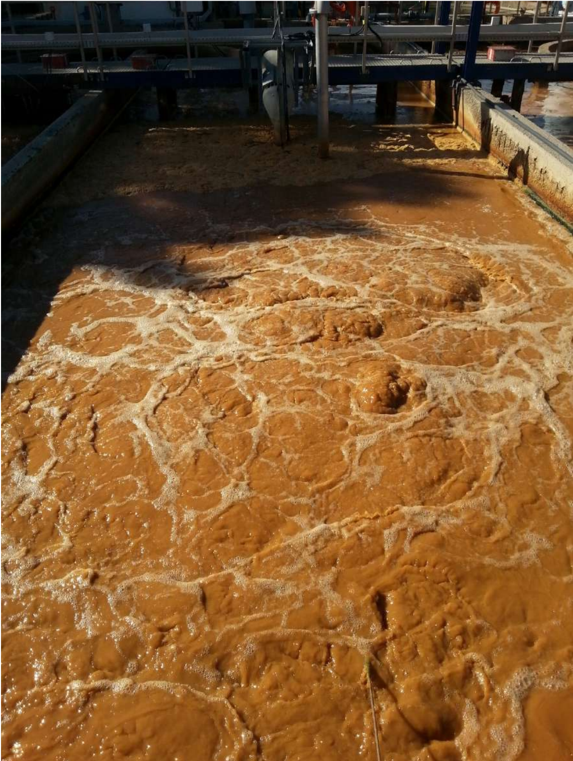
Foto 6 : Optimal agitation inside the tanks to obtain the máximo performance of the biológico depuration process. At the same time that we provide the best oxygenation ratios demanded for the optimal developing of the process. We can observe that there are not foam even fat due to the good function of the primary process of flotation (DAF).
